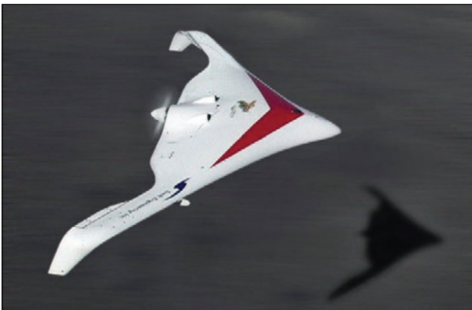
The Swift Engineering KillerBee UAS allows a payload between 14 and 30 kg and can stay airborne for up to 15 hours a useful vehicle for CW detection.
